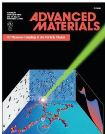
Figure 2.1 – Underlying principle and challenges of self-assembled nanoplasmonics. Laser beam is incident on one end of the complex metal NP network. Optical energy is transported to another end of the network via near-field coupling. Fluorescence of the coupled to metal fluorophore is due to interaction of the transported light with the fluorophore [5]. Inside front cover reproduced with permission of John Wiley and Sons, Inc. All rights reserved.
